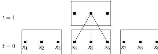
We only need the left and right partition to compute the updated temperature  $x_4$  and  $x_6$ , but we can compute the temperature for  $x_5$  without having the partitions. Thus, we could update the values in the mid of the partition, while waiting to receive the partitions.
