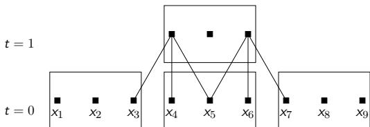
In the previous example we exchanged the whole left and right partition to update the temperatures of the partition in the middle. However, we only need one value of the neighboring partitions to update the temperature for  $x_4$  and  $x_6$ .
