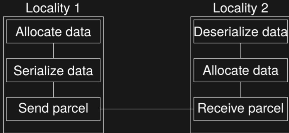
The communication between the localities (nodes) is handled by the so-called parcel port [2]. HPX uses MPI or libfabric for communication between nodes.
