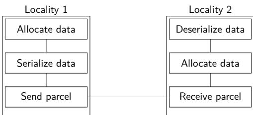
The communication between the localities (nodes) is handled by the so-called parcel port [2]. HPX uses MPI or libfabric for communication between nodes.
