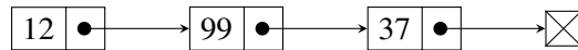
Figure 13.9: A sketch of the linked-list containing three elements. The first pointer points to the second element of the list, the pointer of the second element points to the third element of the list, and the last pointer points to nowhere. This indicates that the end of the list is reached.
