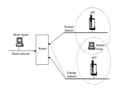
Fig. 3. One-to-one mapping Subnet Architecture testbed
