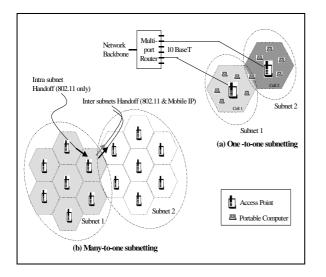
Fig. 2. Mobile-IP based wireless LAN Subnet Architectures
